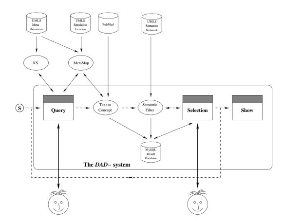
Figure 1: The *DAD*-system. The oval box represents the system itself, everything outside the box represent the resources. The dashed arrowed line indicate the trajectory through the system. See the Architecture section for a full description.
