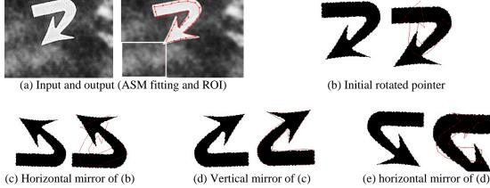
Figure 5. Example of ASM recognition (Left: input to ASM, right: final fitting result with overlaid fitted model)
