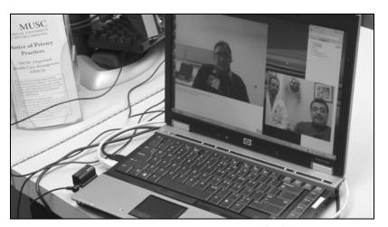
Fig. 1. Laptop with Peripheral Component Interconnect (PCI) cell phone modem at interpretation office.
