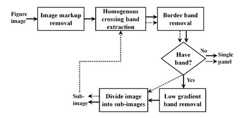
FIG. 4. Process diagram describing the image panel segmentation procedure.
